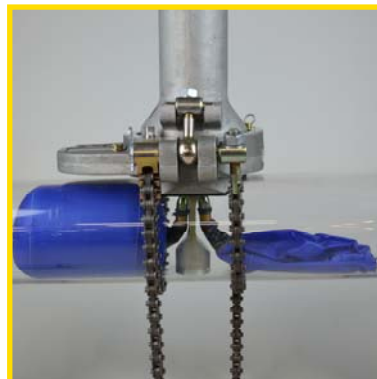
Twin Bagtube flowstopping inflation process
